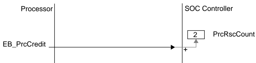
Figure 8-6 Processor Resource Control
